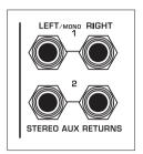
Fig. 2.8: Stereo aux return connectors
